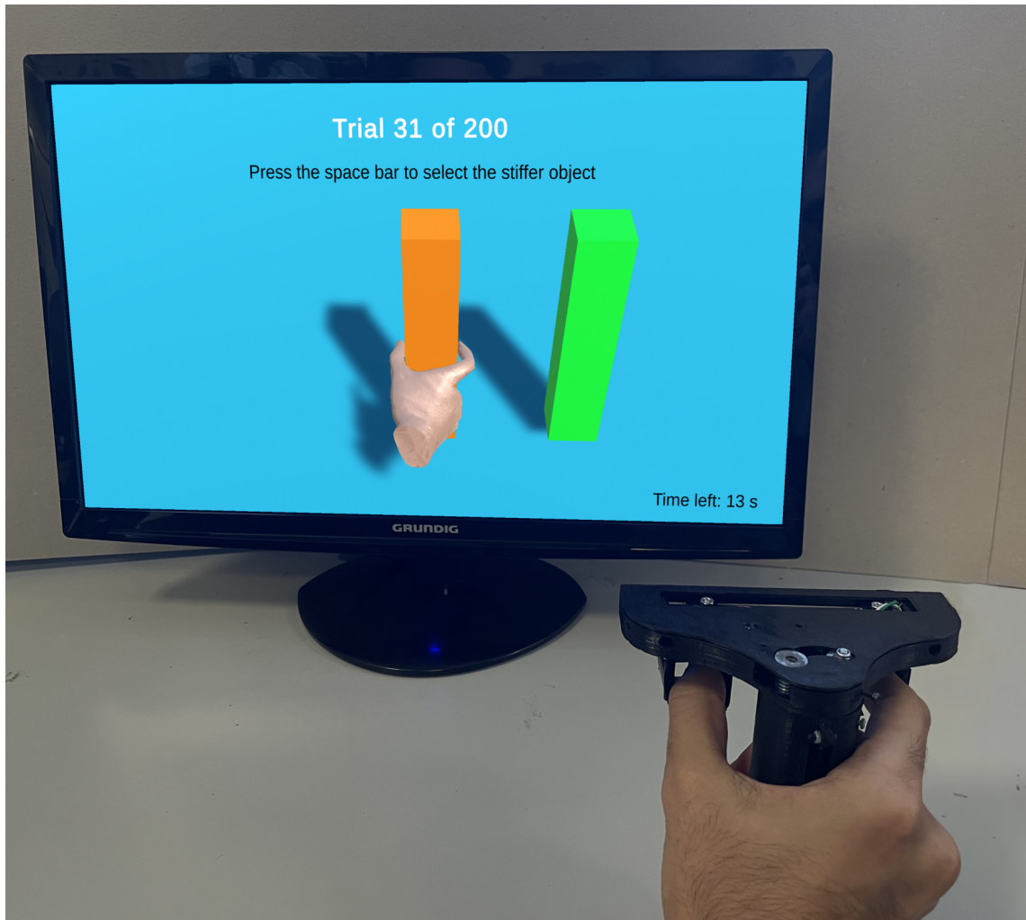
Figure 3.1: In the force stretch feedback experiments, two virtual objects are displayed side by side on the computer screen. The participants are asked to select the stiffer object by squeezing them. Participants had 15 seconds to answer each trial (they were given another 15 seconds if they could not answer within the first 15 seconds, which resulted in zero unanswered trials). Note that the device and the holding hand are covered with a cardboard box during the experiments.
